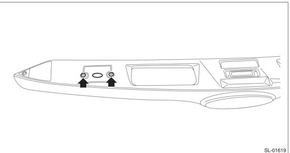
3) Release the locks at both ends of the button - opener rear gate by pushing them with a flat tip screwdriver, remove the button - opener rear gate and remove the integrated harness.
